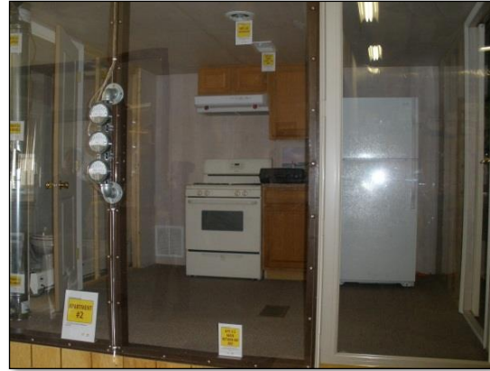
Figure C1.4. At AEA's training facility, kitchen mock-up for CO testing on gas range and fridge metering
